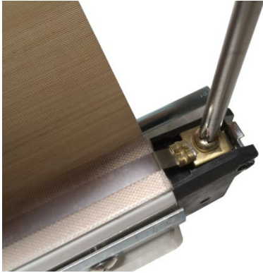
Figure 3. Screw element in place.
