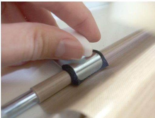
Figure 5. Loosen multi-star knob to remove the PTFE roller.
