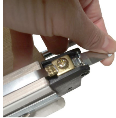
Figure 4. Lift latch on heating block to screw element in place.
